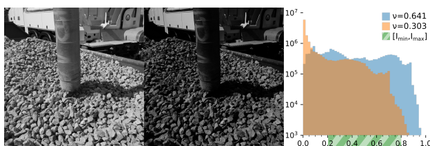
Figure 3. A well-lit image (left, blue histogram) has a stronger presence in the preferred intensities range of the linear pixel intensities histogram (right, green) in comparison to the underexposed image (middle, orange histogram). This is reflected in a higher fitness score \nu for a well-lit image.
